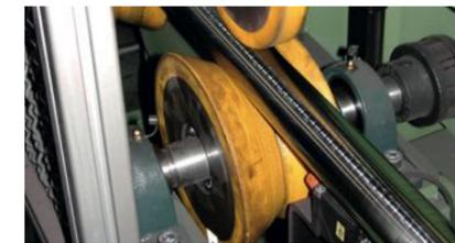
Guide and pressure rolls with exchangeable cores
